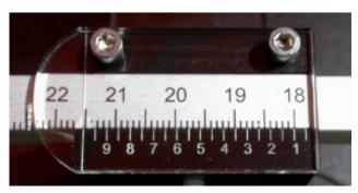
This is 215,25 mm P2S - for the DaVinci 9" tonearm. Note that the white line between "2" and "3" in in-line with the black line above on the aluminum scale. This means 215 mm PLUS 25/100 mm. Resulting in 215,25 mm P2S. The vernier scale "adds" the 5/100 mm value to the full mm read-out on the large metric scale.
